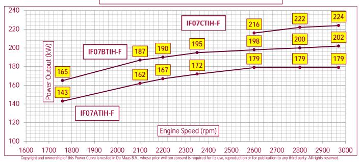
Although our FM ratings are shown at specific speeds, De Maas FFE engines can be applied at any intermediate speed. To determine the intermediate speed power; make a linear interpolation from the applicable De Maas power curves.
