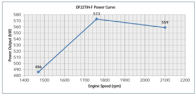
Although our FM ratings are shown at specific speeds, De Maas FFE engines can be applied at any intermediate speed. To determine the intermediate speed power; make a linear interpolation from the applicable De Maas power curves.
