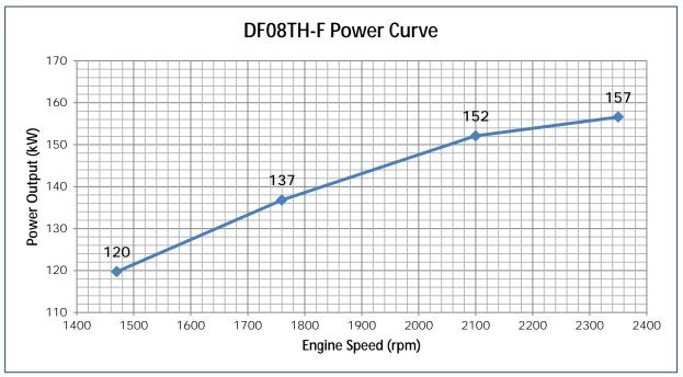
Although our FM ratings are shown at specific speeds, De Maas FFE engines can be applied at any intermediate speed. To determine the intermediate speed power; make a linear interpolation from the applicable De Maas power curves.
